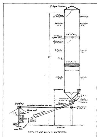
fig. 5. One of the first 10-meter rotary beam antennas was used at W6JN. Composed of three half waves in phase with reflectors, the array was suspended from a wooden telephone pole. It probably provided gain equivalent to today's 3-element Yagi. In 1936 when large beams on 10 meters were unknown, it must have been a block-buster! (Drawing reproduced from the April, 1936, issue of QS7).
